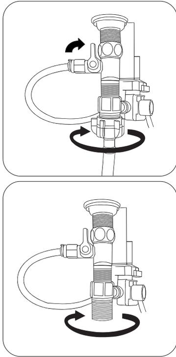
**2** The water filter is located inside the 7/8" adaptor. Gently remove it and gently brush it with a toothbrush to remove any residue. Place the filter back inside the adaptor.
