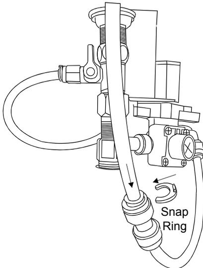
Pull out the snap ring from the connector. Firmly push the bidet water tank tube protruding behind the toilet inside the pressure connector. Then re-insert the snap ring.
