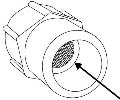
**3** Reconnect the 7/8" adaptor and the water supply line to the toilet's water inlet. Open the ball valve at the back of the toilet.
