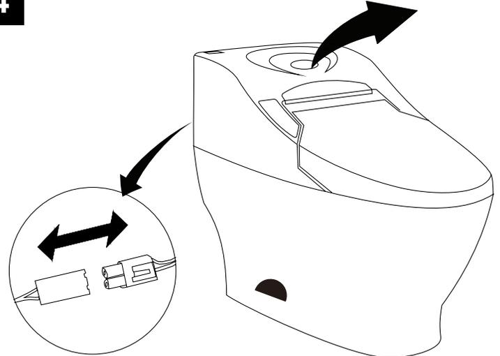
Make sure that the electronics plug behind the toilet is unplugged. Then remove the seat from the ceramic base. Simply pull the seat up gently. Be careful.
