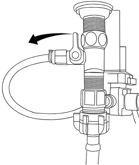
Ensure that the ball valve at the back of the toilet is open. Open the water inlet valve and check for leaks.
