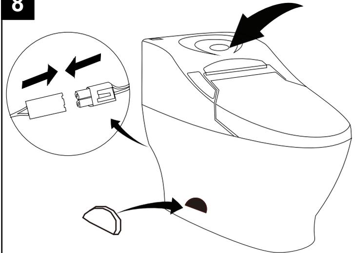
With care, re-install the seat on the ceramic base and connect the electrical plug at the back of the toilet. Then cover the side holes with the supplied covers.
