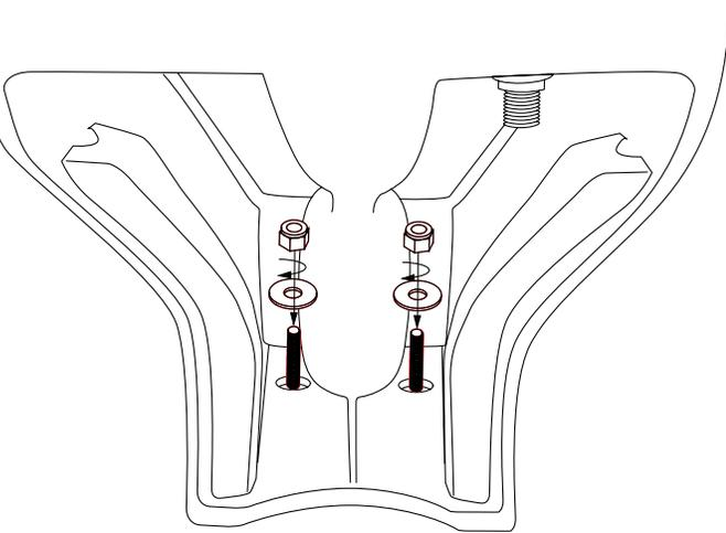
Using a wrench, install the washer and the nuts of the flange bolts through the toilet's side holes. Tightly screw the nut to secure the toilet.
