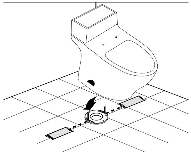
Position the toilet on the floor flange, making sure the fixing bolts are aligned with the toilet's holes.
