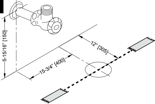
Ensure that your water inlet pipe and your floor discharge drain are installed according to the drawing. These are minimum measurements, the toilet can be installed if your actual measurements are longer than shown.
