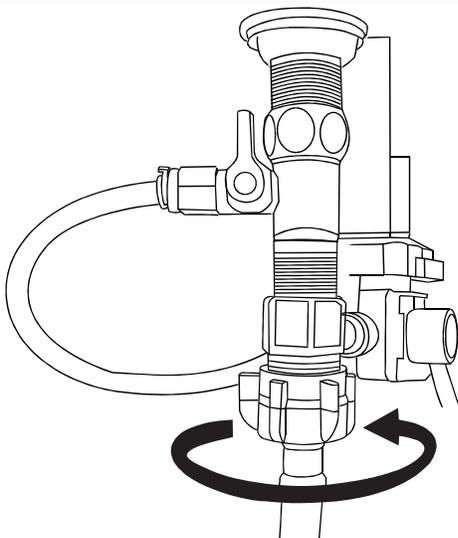
Connect the provided supply line to the water inlet located at the back of the toilet.
