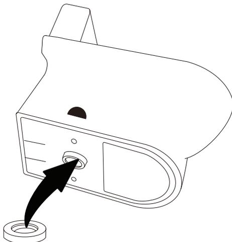
Firmly push the seal ring onto the toilet's drain, fixing the seal ring to the ceramic.
