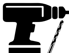
Drill and drill bits Perceuse et forets Taladro con brocas ø3/16" (5mm)
