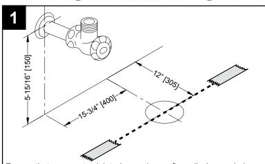
Ensure that your water inlet pipe and your floor discharge drain are installed according to the drawing. These are minimum measurements, the toilet can be installed if your actual measurements are longer than shown.
