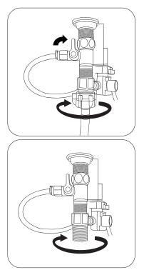
The water filter is located inside the 7/8" adaptor. Gently remove it and gently brush it with a toothbrush to remove any residue. Place the filter back inside the adaptor.
