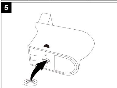
Firmly push the seal ring onto the toilet's drain, fixing the seal ring to the ceramic.
