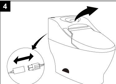
Make sure that the electronics plug behind the toilet is unplugged. Then remove the seat from the ceramic base. Simply pull the seat up gently. Be careful.
