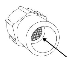
Reconnect the 7/8" adaptor and the water supply line to the toilet's water inlet. Open the ball vavle at the back of the toilet.
