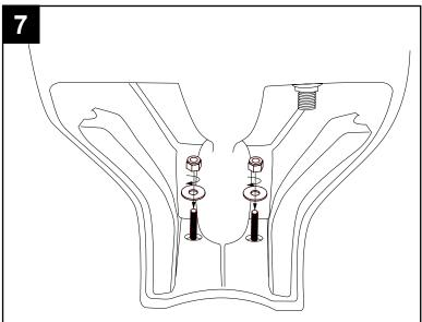
Using a wrench, install the washer and the nuts of the flange bolts through the toilet's side holes. Tightly screw the nut to secure the toilet.
