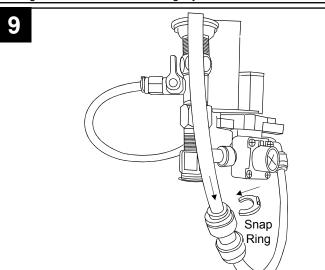
Pull out the snap ring from the connector. Firmly push the bidet water tank tube protruding behind the toilet inside the pressure connector. Then re-insert the snap ring.
