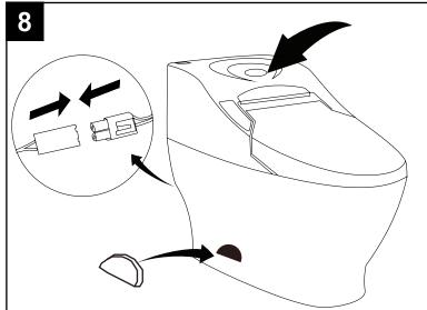
With care, re-install the seat on the ceramic base and connect the electrical plug at the back of the toilet. Then cover the side holes with the supplied covers.
