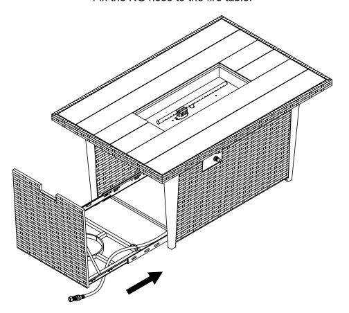
Install the NG hose to the fire table using wrench.
