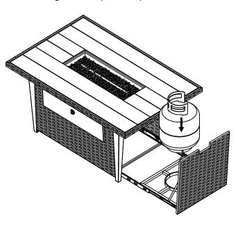
Secure the gas tank to the fire table at the bottom using the bolts. Connect the gas to the fire table using LPG regulator.
