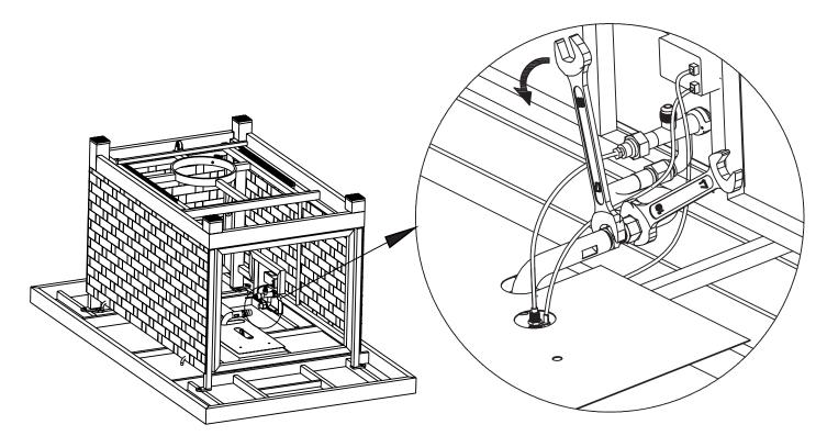
Disconnect the pipe and the LPG reducer.
