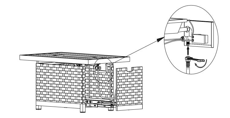
Install the NG hose to the NG inlet of fire table using wrench.
