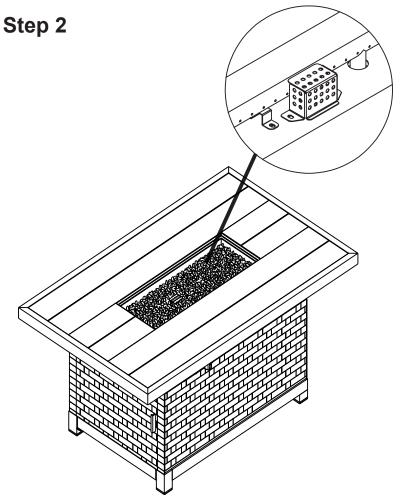
Put the glass beads onto the burner.
