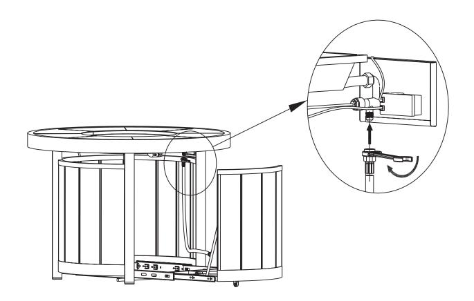
Install the NG hose to the NG inlet of fire table using wrench.
