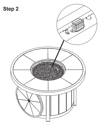
Put the glass beads onto the burner.
