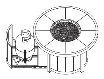
Secure the gas tank to the fire table at the bottom using the bolts. Connect the gas to the fire table using LPG regulator.
