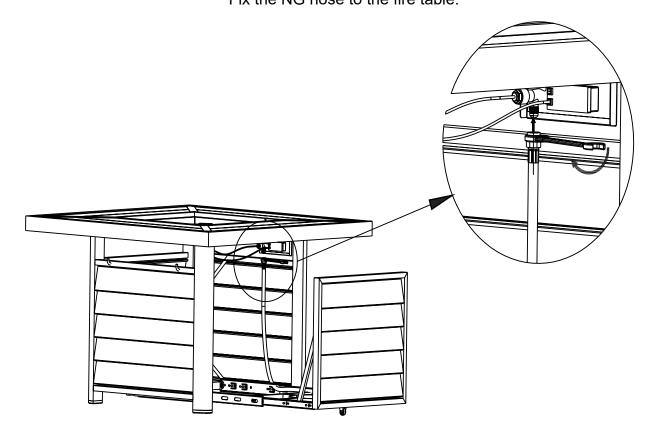
Install the NG hose to the NG inlet of fire table using wrench.
